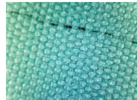
Polyester filament fiber containing carbon fiber
